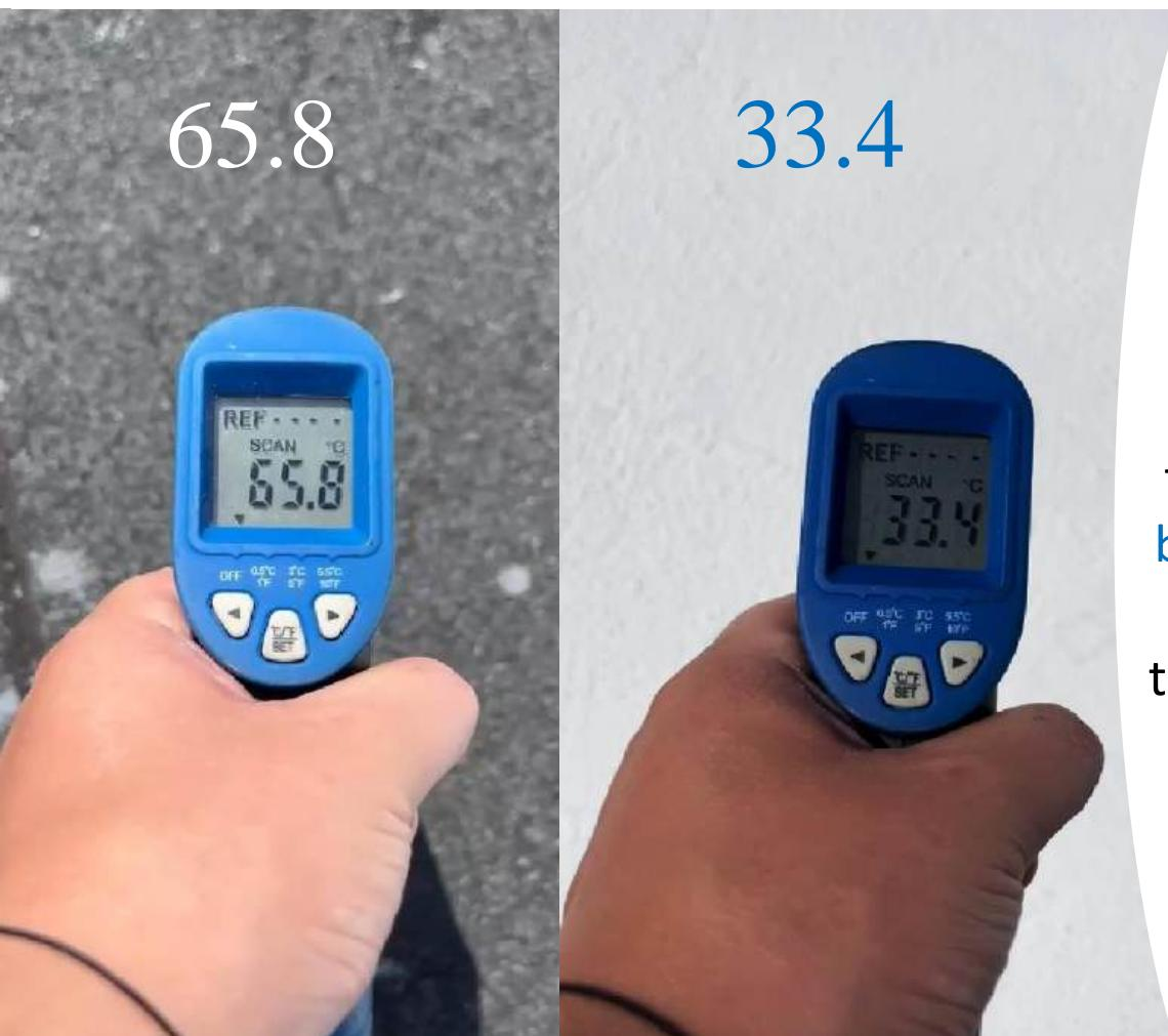
The SMART system lowers the roof temperature by up to 70%, making it up to 10°C cooler under the roof on hot days.
